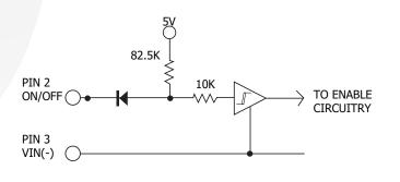
Figure B: Internal ON/OFF pin circuitry
